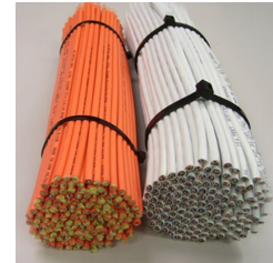
Conventional Cable 144 Multimode Fibers 144 Copper Cable
